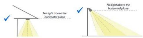
*horizontal plane*, in relation to a light fitting, means the horizontal plane passing through the centre of the light source (for example, the bulb) of the light fitting. *outside light fitting* means a light fitting that is attached or fixed outside, including
